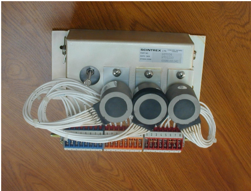
Reactor Trip Switch, Rear View
